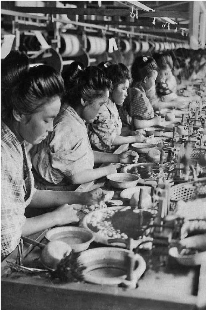
Japan. Silk factory girls drawing thread from cocoons (photo T. Enami; www.flickr.com/photos/okinawa-soba/albums/7215762339925022 ). Cocoons are inserted into the hot water, where the machine finds several threads and the ends of fibers winds into threads. Over time, the machines were converted to fully automatic.
