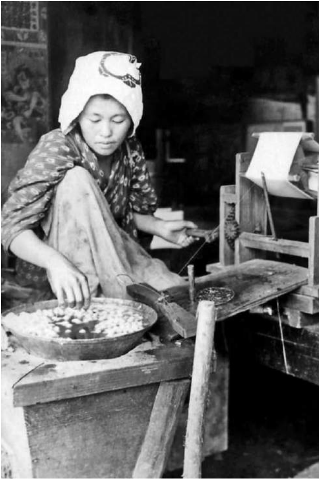
Japan. Wooden gears wind the raw silk strands from cocoons (photo T. Enami; www.flickr.com/photos/okinawa-soba/albums/7215762339925022 ). Women insert cocoons in a bowl of hot water, wind and twisted fiber with right hand while the left hand spiraled coil winding.
